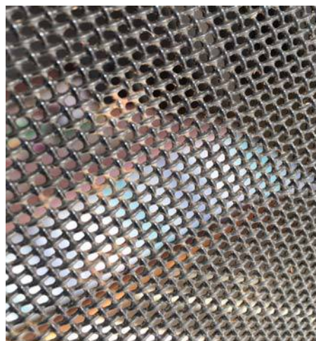
Close up of dirt build up on woven S.S. mesh
